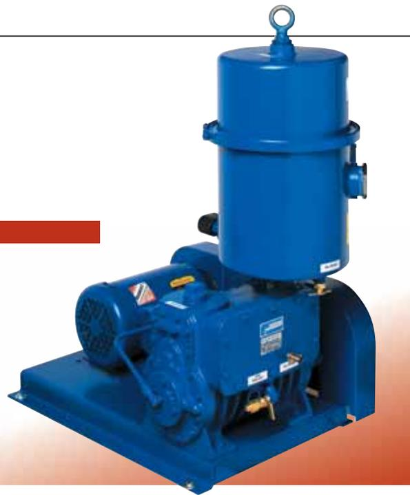
These are other quality features: a controllable gas ballast to permit the handling of condensable vapors and to minimize oil changes due to vapor contamination of the sealing oil. Models KD-30 and KD-50 are equipped with an oil mist eliminator, optional on model KDH-130 & KDH-150. Each pump operates within the rating of its standard TEFC motor throughout the entire operating pressure range.
