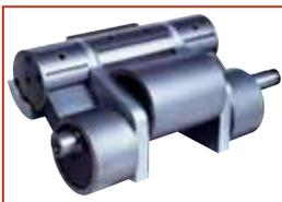
Kinney KT Pumps have three sets of cams and pistons driven by a common shaft. One cam and piston set is no longer than the other two and the cams are set 180° apart. The dynamic forces produced by the rotation of the long cam
