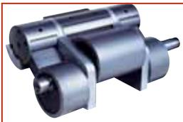
Kinney KT Pumps have three sets of cams and pistons driven by a common shaft. One cam and piston set is no longer than the other two and the cams are set 180° apart. The dynamic forces produced by the rotation of the long cam
