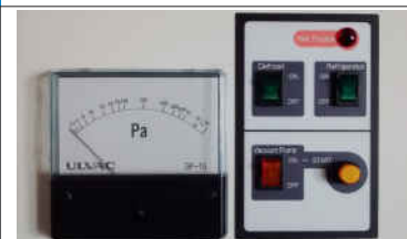
Pirani Vacuum Gauge and Control Panel
