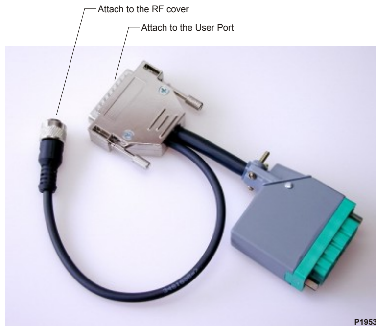
Figure 5-5. RF / User Port interlock adapter cable
