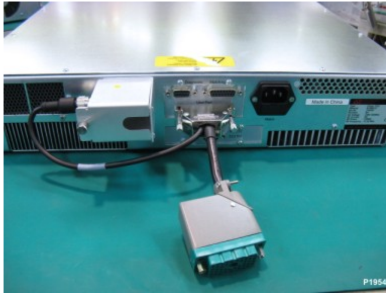
Figure 5-6. RF / User Port interlock adapter cable, attached to unit
