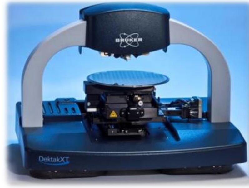
Auto X-Y-Theta Stage with 8" wafer vacuum chuck
