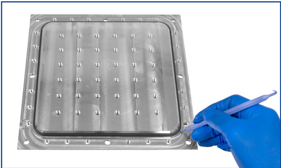
Figure 5 - Remove the O-ring from the groove
