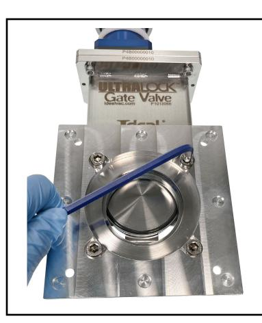
Get a metric hex wrench (6 or 8 mm) and metric screws out of the adapter kit.
