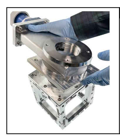
Place the valve on to the Cube with the mounted adapter plate face down.
