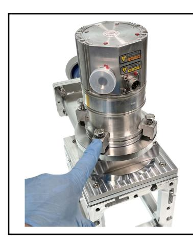
Note: The gate valve has an ISO-F flange with metric tapped holes. The turbo pump has an ISO-K flange.
