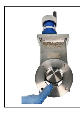
Open the gate valve slightly to determine which side of the gate the O-ring is on.
