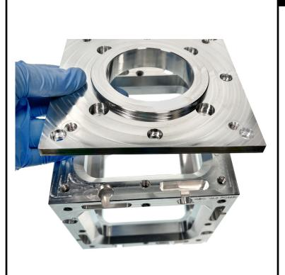
Orient the Cube so that the face that will receive the gate valve is up.
