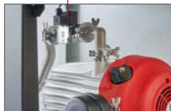
Backing pump with backing vacuum safety valve
